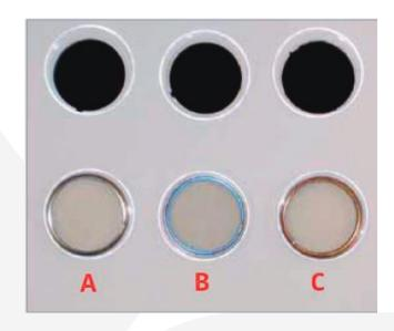
The top row shows the filter soot emissions in conventional units; measured soot concentration 43.4 mg/m³. The bottom row shows the filter soot emissions with use of ClearAir particulate filter; measured soot concentration of <0.01 mg/m³.
